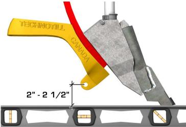
• The opener may need to be shimmed at either the top or bottom shank bolt to ensure the point is properly positioned in relation to the packer plate.
