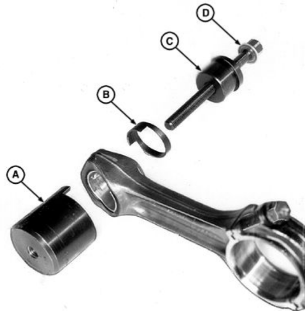
Removing Piston Pin Bushing from Rod
