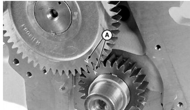
Timing Marks—Camshaft and Crankshaft Gears
