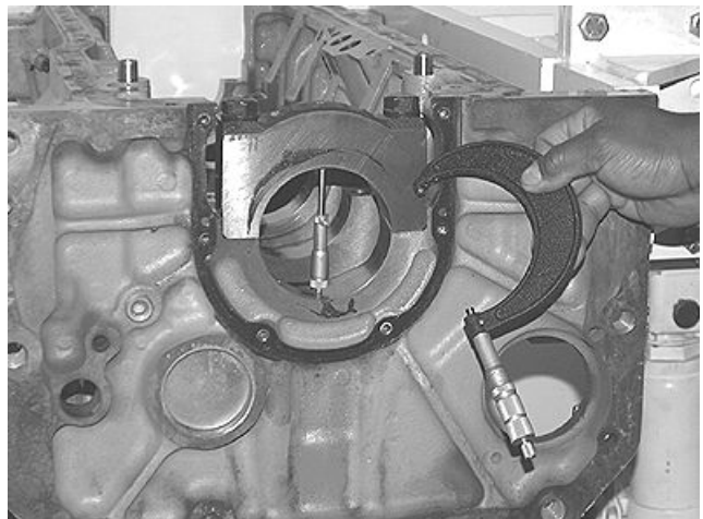
Measuring Main Bearing Cap Bores
