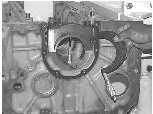
Measuring Main Bearings
