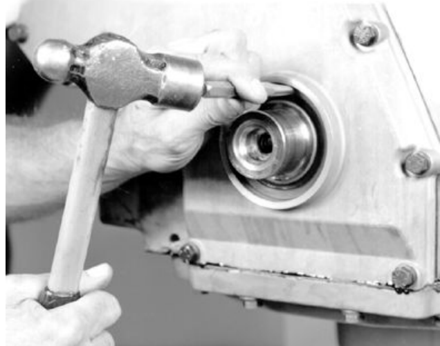
Center Punching Front Oil Seal Casing
