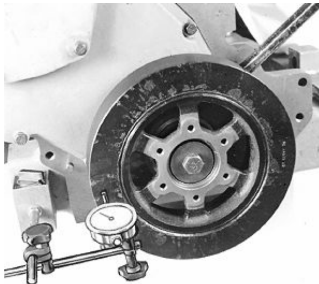
Checking Crankshaft End Play
