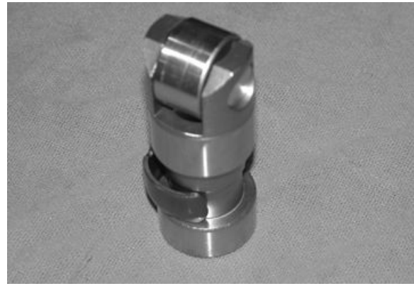
Inspect Roller Follower
