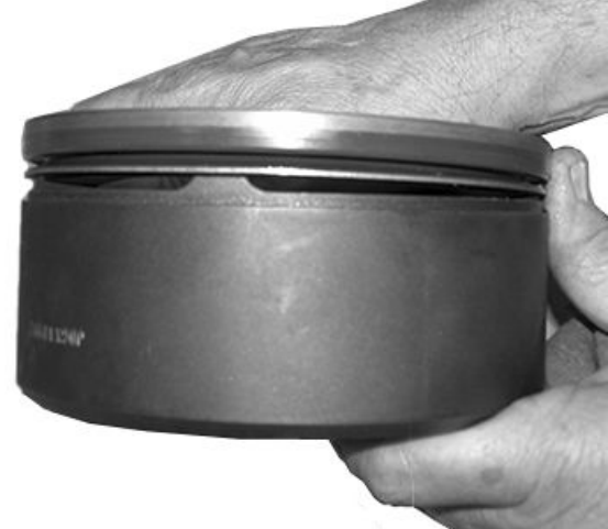
Raised Notch on JDG10997 Seal Driver
