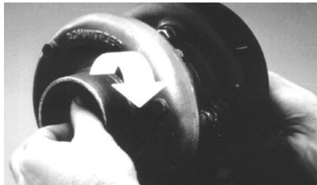
Checking Shaft Rotation and Clearance
