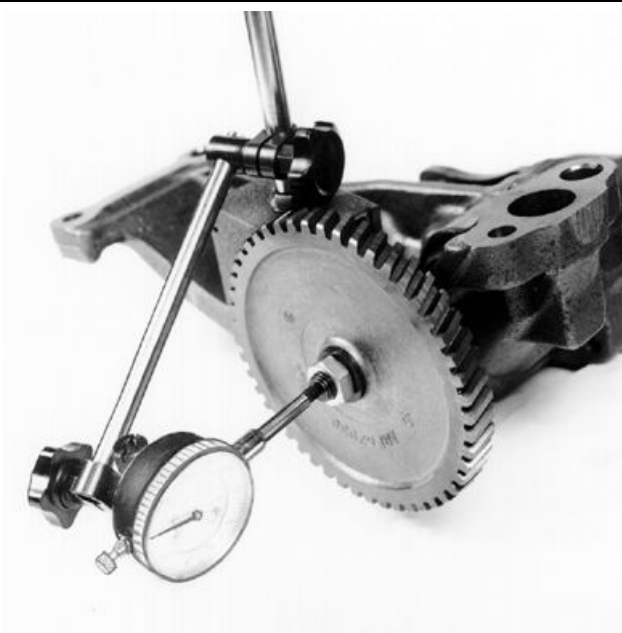
Checking Pump Shaft End Play
