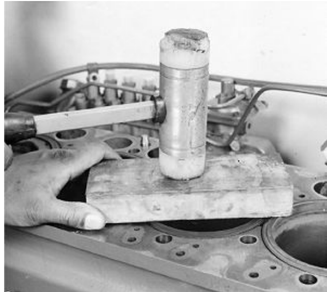
Seating Cylinder Liners in Block
