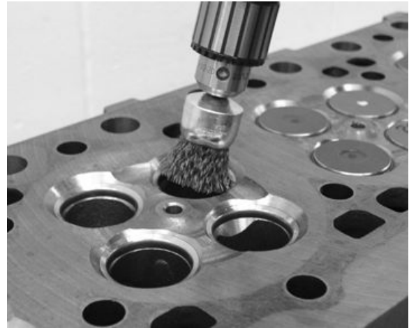
Cleaning Valve Seats
