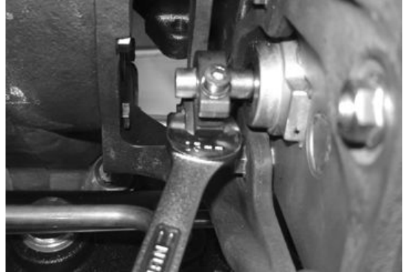
Using Wrench to Support Linkage
