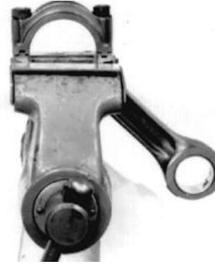
Clamping Rod in Vise
