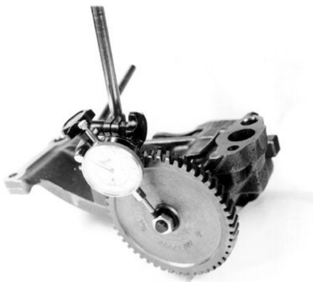
Checking Pump Shaft Side Movement
