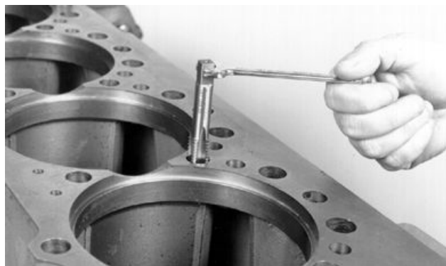
Tap for Head Mounting Holes in Block
