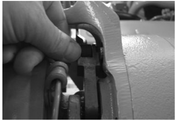
Check for Linkage Free Travel
