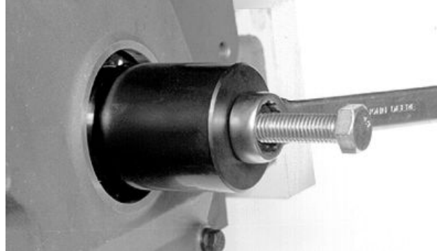
Installing Puller to Remove Front Wear Sleeve
