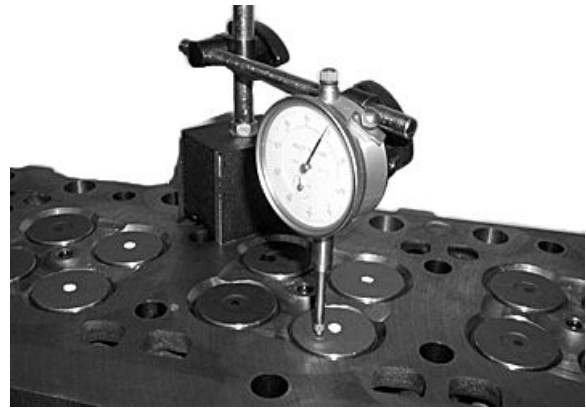
Measuring Valve Recess
