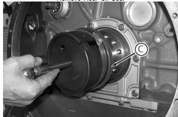
Oil Seal Removed from Engine
