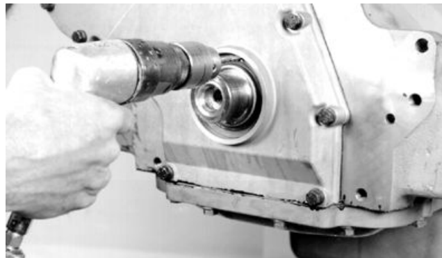
Drilling Hole in Front Oil Seal Casing
