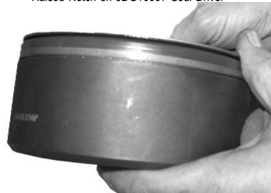
Rear Seal Properly Fitted to Seal Driver
