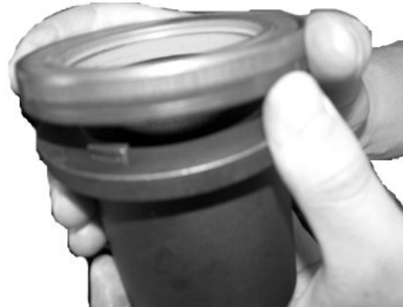
Raised Notch on JDG11004 Seal Driver
