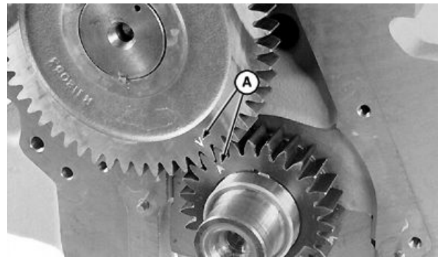
Timing Marks—Camshaft and Crankshaft Gears
