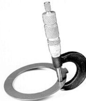
Measuring Camshaft Thrust Washers
