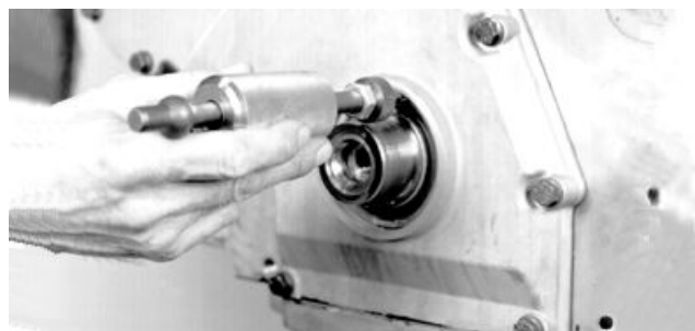
Removing Front Oil Seal
