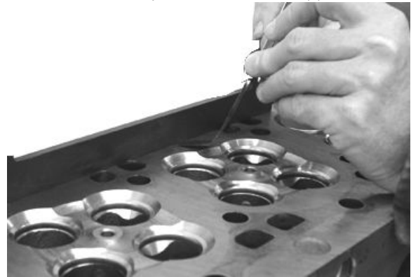
Check Cylinder Head Flatness (2)
