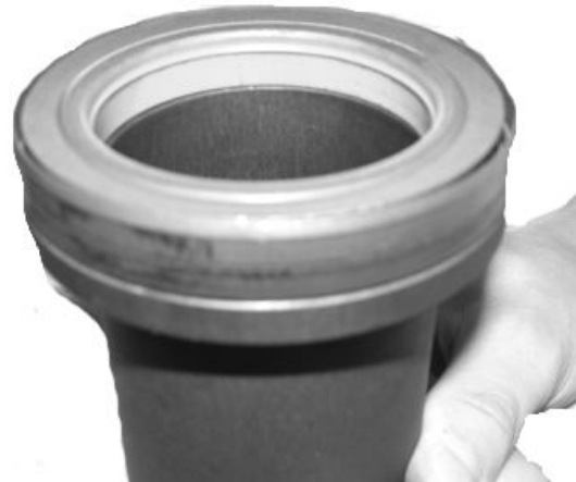
Seal Properly Fitted to Installation Tool
