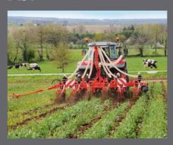
An incorporator provides fertilizer at a constant depth in order to fertilize:
