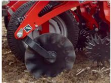
The wavy disc provides improved soil expansion before the tine's passage. It is recommended for use following a fasciate-rooted crop (ray-argss)
