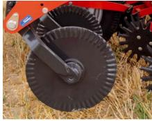
**The disc** opens the way for the tine and cuts plant residues.
